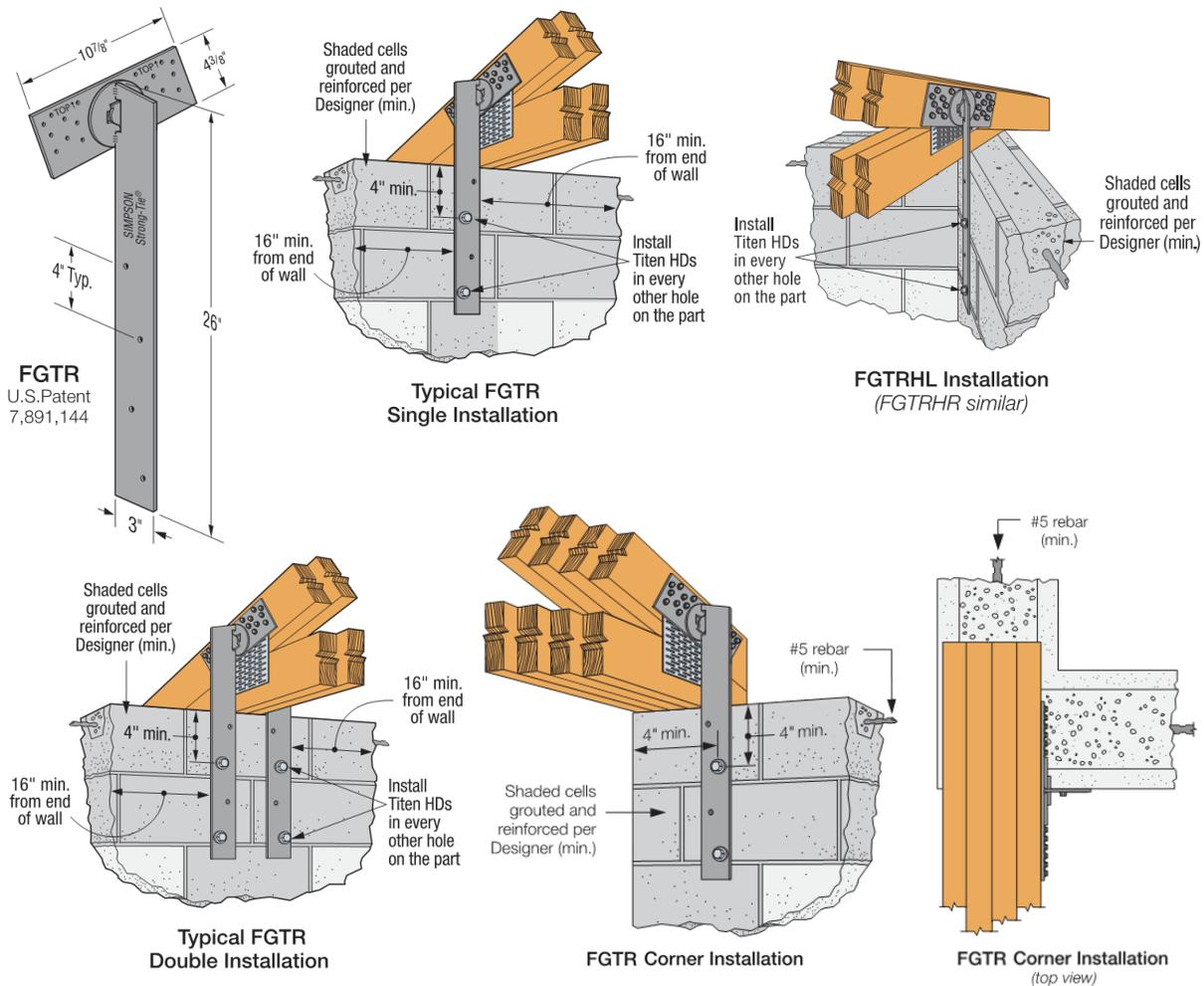
FIGURE 6: FGTR / FGTRHL / FGTRHR Dimensions and Installation Details
