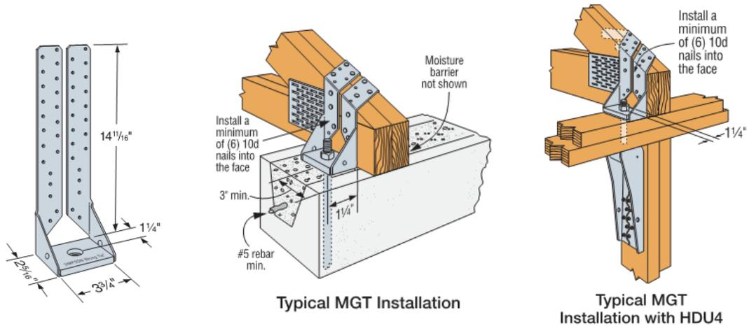
**FIGURE 9: MGT Dimensions and Installation Details**
