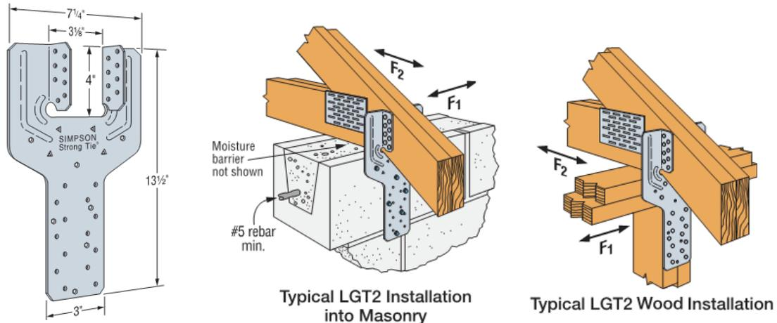
FIGURE 7: LGT2 Dimensions and Installation Details
