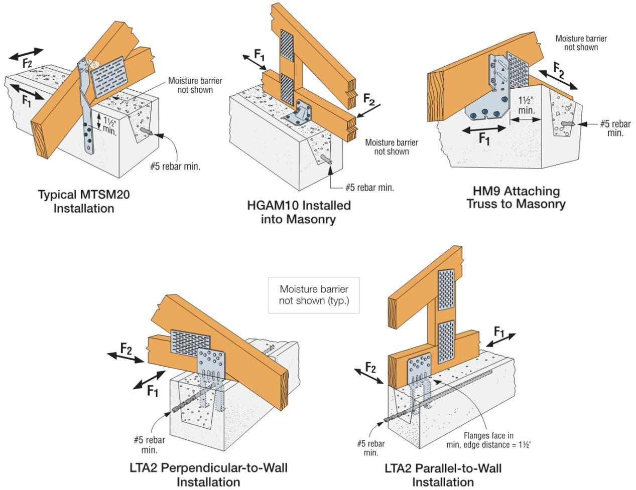
**FIGURE 2: MTSM / HTSM / HM9 / HGAM10 / LTA2 Installation Details**
