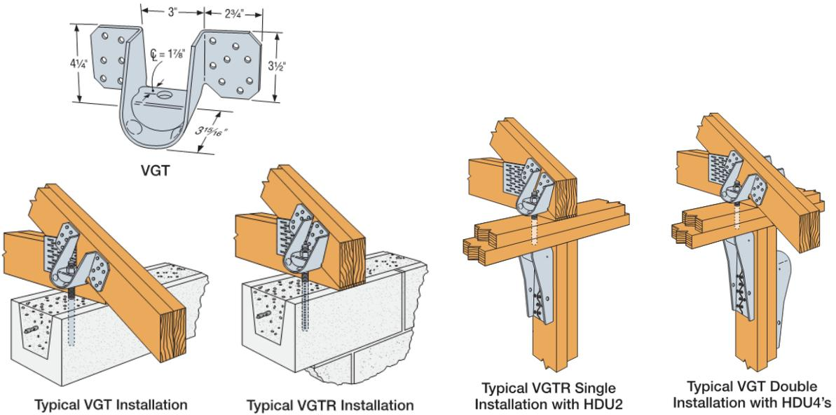
**FIGURE 10: VGT / VGTR / VGTL Dimensions and Installation Details**
