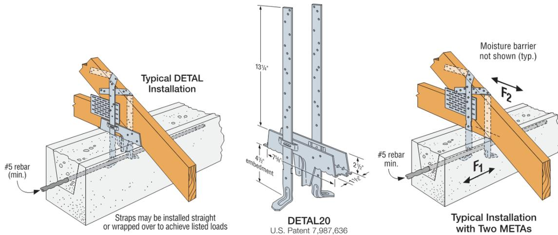
FIGURE 4: DETAL20 Dimensions and Double META / HETA / HHETA Installation Detail
